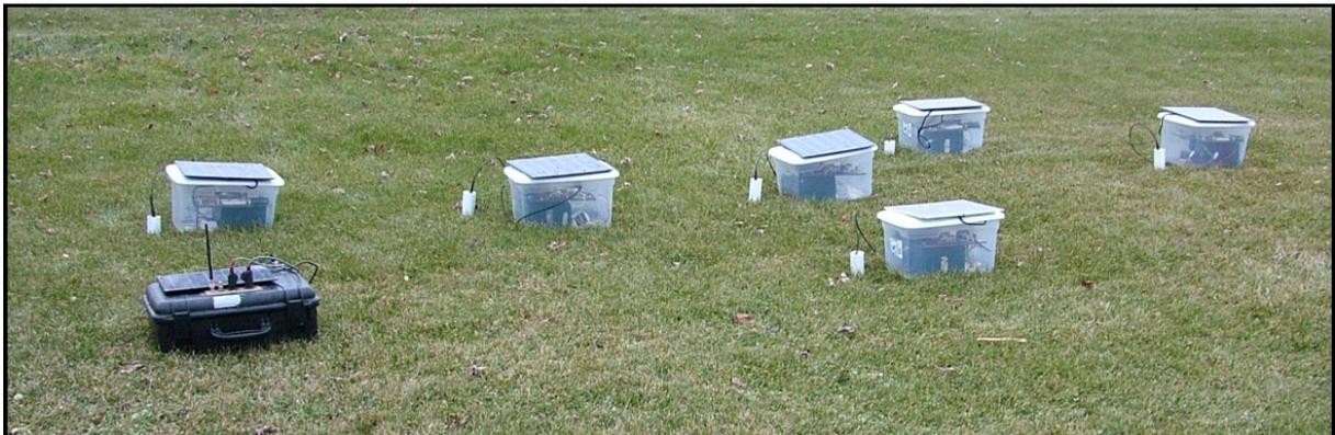
Figure 32 Experimental setup. Only the antennas were installed below the surface of the ground at a depth of 80 cm. The antennas were lowered into PVC tubes driven into the ground. Motes were sealed from the elements inside of plastic containers. CS616 soil moisture probes monitored soil conditions between links. Data consisted of RSSI and soil moisture between all links. All data was routed and stored at the base station that consisted of custom data logger designed for this experiment.
