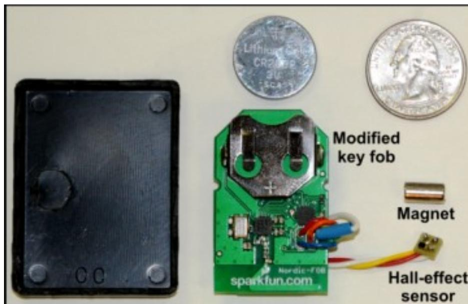
Figure 17 Off-the-shelf modified key fob with low power Hall-effect sensor that was attached to mussel.
