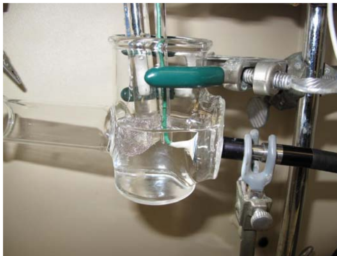
Figure 6. A photograph of a cell set up. A semiconductor electrode (green wire) is facing the fiber optic light guide. The fiber optic light guide is touching the window of the cell while the SE is placed at the blue line on the apparatus glass to fix the distance between them.
