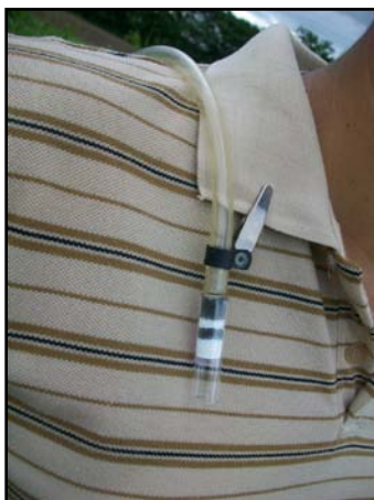
Figure 4.1 Study participant equipped with OSHA Versatile Sampler (OVS-2) sorbent tubes.
