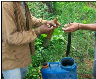
Figure 4.5 Dismantling and repairing the nozzle of a backpack sprayer that had become clogged because of debris in the water.
