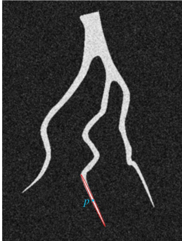
Figure 4.2: A schematic representation of a vascular tree structure in 2D. Tensor scale at a point p is indicated by the ellipse in red. The proposed constrained region growing algorithm uses this knowledge to facilitate growth along the structure while restricting growth across the local structure to stop leaking.
