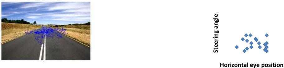
Figure 9. Glance locations and hypothetical scatter plots of associated horizontal eye position and steering wheel angle for non-distracted and distracted driving on a straight road
