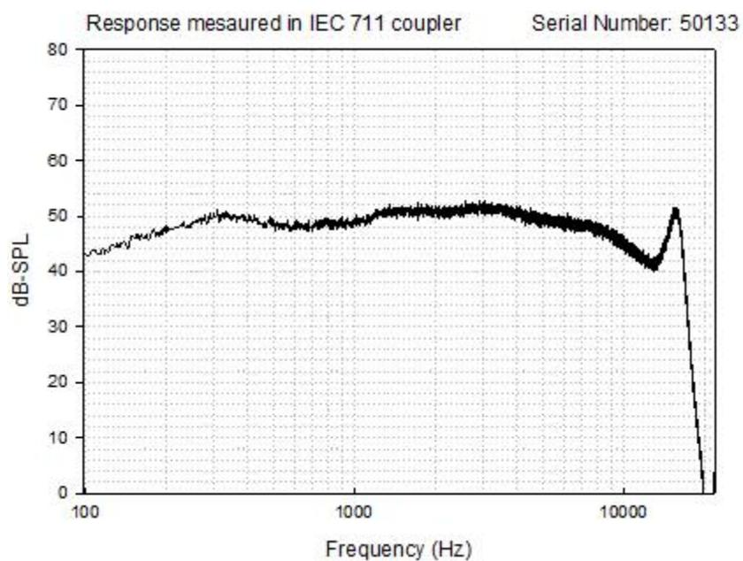
Figure A2. The frequency response of the right insert earphone.
