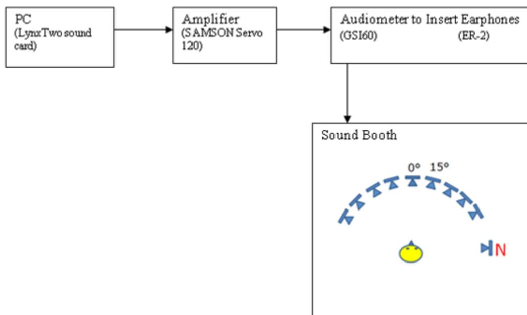
Figure 4. Experimental set-up diagram.
