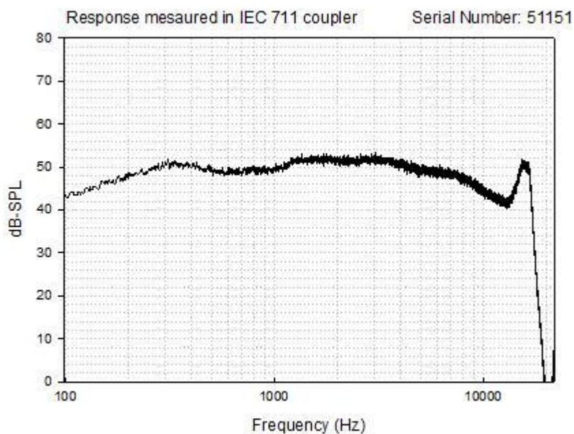
Figure A1. The frequency response of the left insert earphone.
