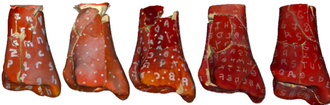
Figure 50 Although some dusting was observed at the most proximal segment of the tibia, the articular and metaphyseal bone volume was preserved during impact. Subsequently, the 5 replica tibias were accurately reconstructed by matching native surfaces to the pre-fractured template.
