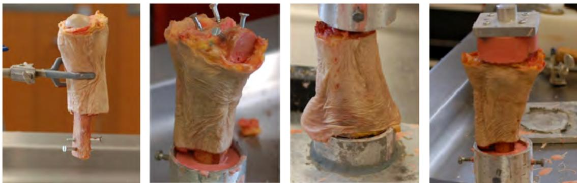
Figure 19 The process of preparing the cadaveric specimen is shown. With the joint capsule intact, the proximal shaft of the tibia and the inferior talar surface were potted in PMMA. A steel platen for impactation was attached to the talar side.
