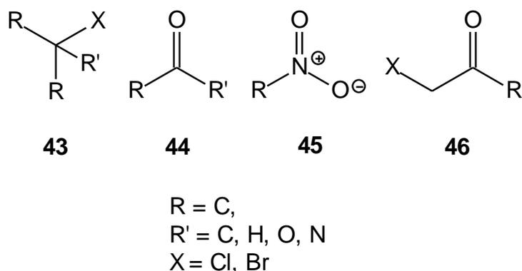
Figure 15. Structures not well tolerated in the Arbuzov reaction.
