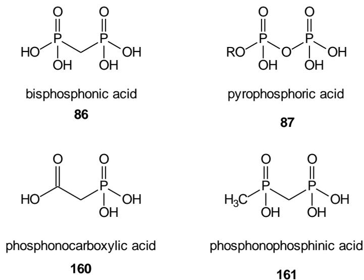
Figure 50. Pyrophosphoric acid and bioisosteres.
