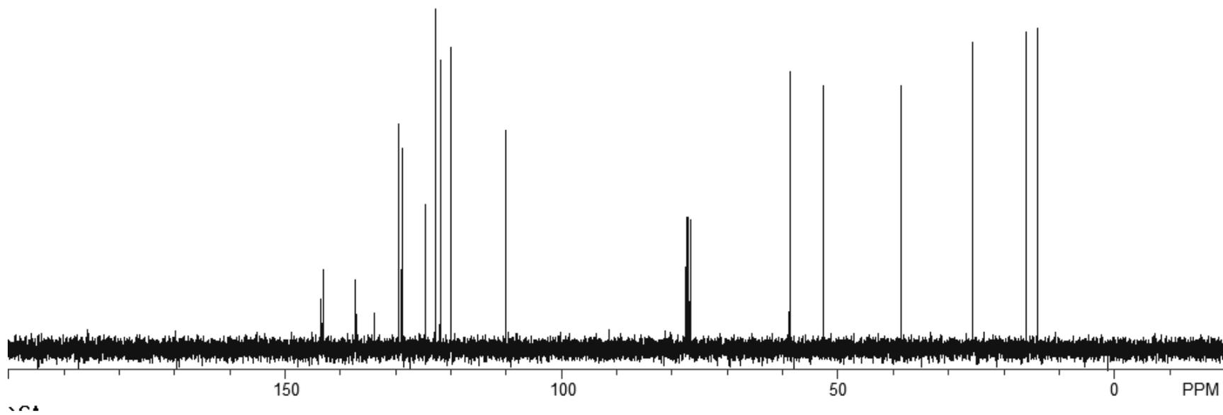
Figure A69.  $^{13}\text{C}$  NMR spectrum for alcohol **195**.
