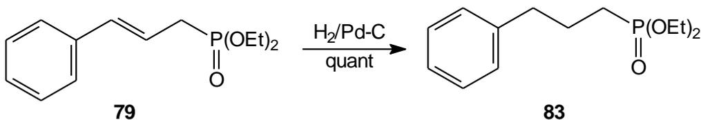
Figure 25. Synthesis of an aliphatic phosphonate via catalytic hydrogenation.
