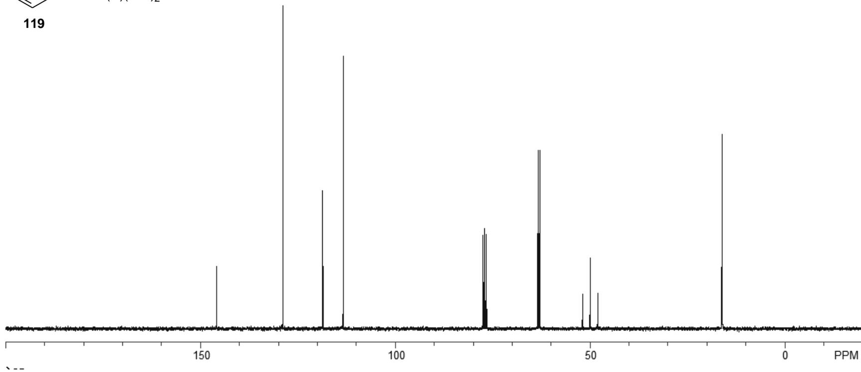
Figure A14.  $^{13}\text{C}$  NMR spectrum for bisphosphonate **119**.
