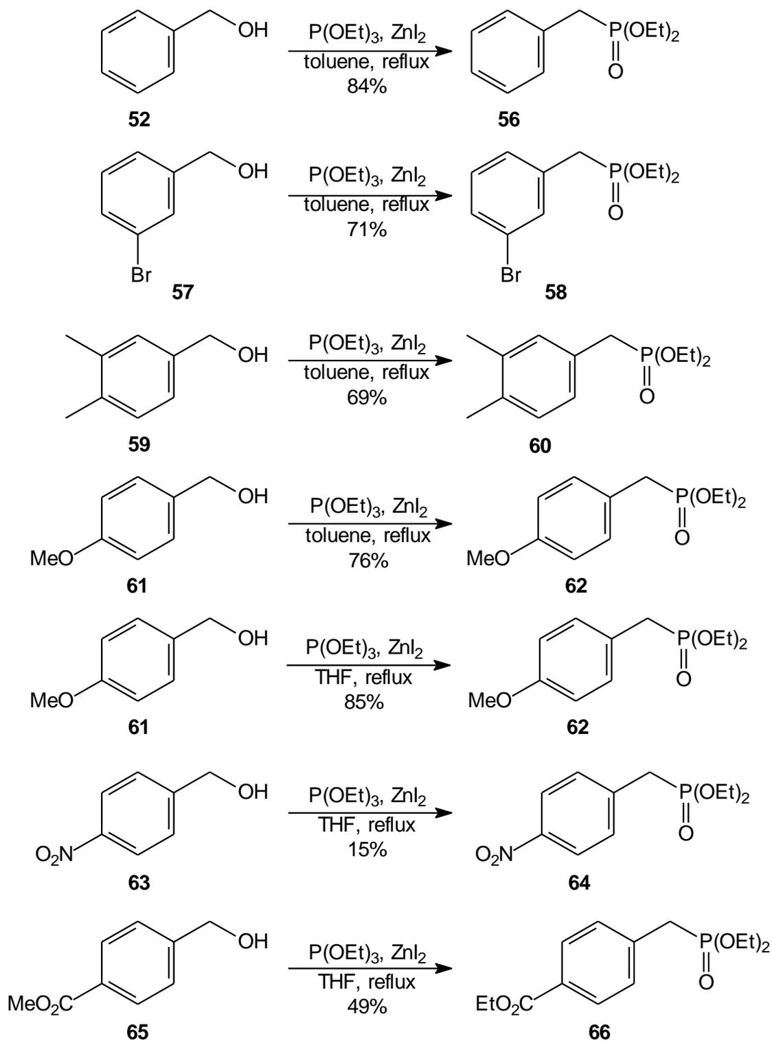
Figure 20. Zinc iodide mediated phosphonylation of benzylic alcohols.
