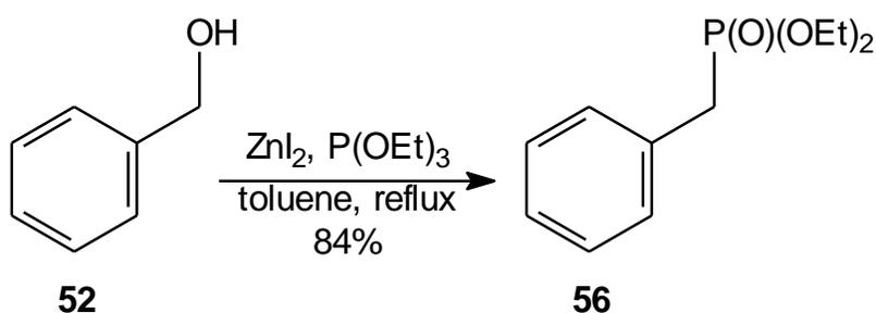
Figure 19: The conversion of benzyl alcohol to diethyl benzylphosphonate (**56**).
