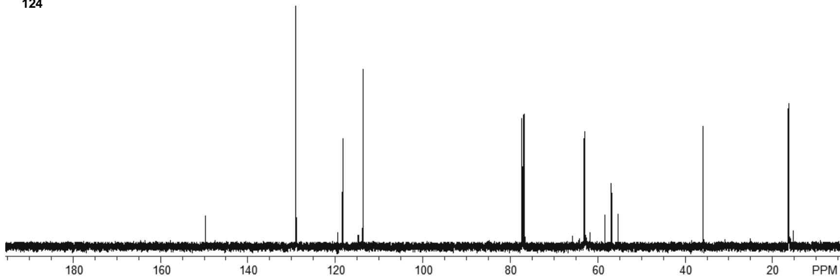
Figure A19.  $^{13}\text{C}$  NMR spectrum for bisphosphonate **124**.
