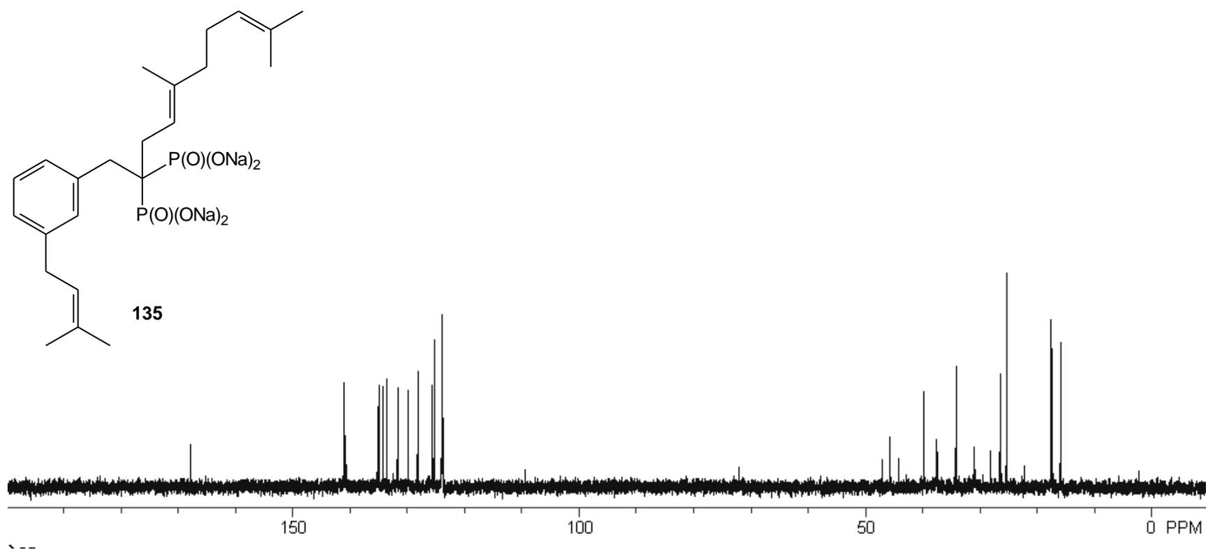
Figure A31.  $^{13}\text{C}$  NMR spectrum for bisphosphonate **135**.
