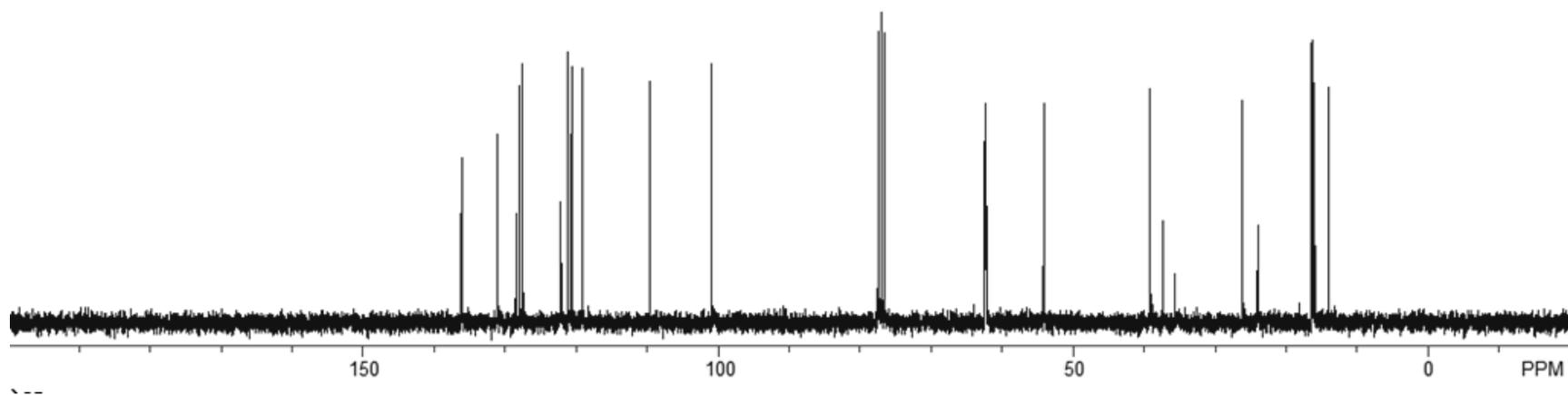
Figure A65.  $^{13}\text{C}$  NMR spectrum for bisphosphonate **193**.
