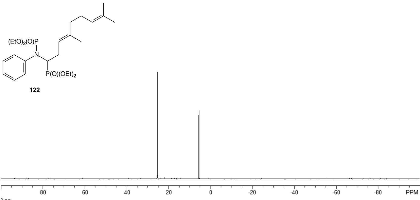
Figure A17.  $^{31}\text{P}$  NMR spectrum for compound **122**.
