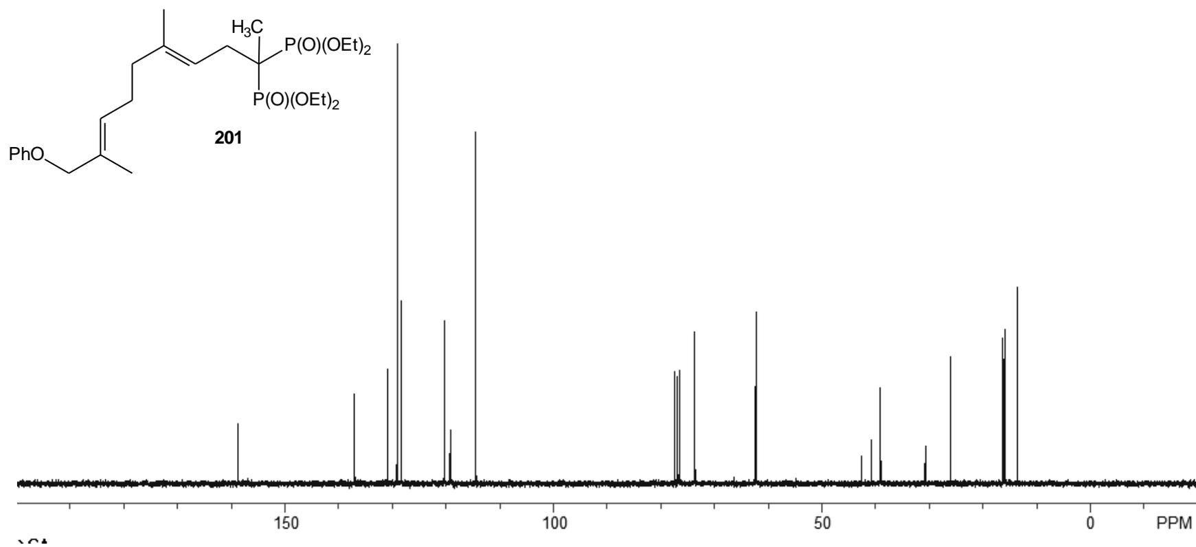
Figure A71.  $^{13}\text{C}$  NMR spectrum for bisphosphonate **201**.
