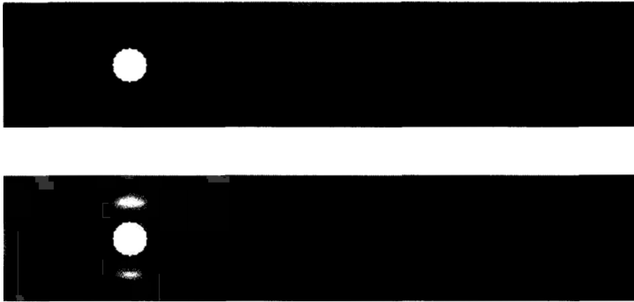
Figure 2.1: Flow through a Karman channel in the Stokes regime (laminar flow, Re = 1 , bottom) and intermediate regime (Karman vortices, Re = 200 , top). Colours indicate the absolute velocity |\mathbf{u}| .
