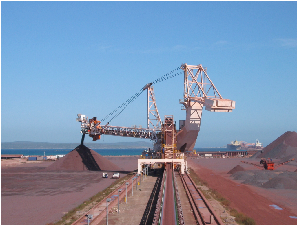
Figure 8.4: A Stacker/Reclaimer depositing ore onto a stockpile in the Port of Saldanha 4 .
