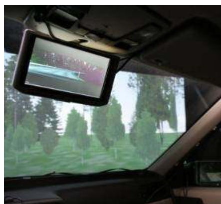
Figure 4. (a) VTI moving-base driving simulator. (b) simulator vehicle chassis (Volvo 850). (c) wide-angle visual screen with 120° horizontal field of view. (d) visual projection system. (e) left outside mirror (monitor). (f) rear mirror (monitor) and right outside mirror (monitor).
