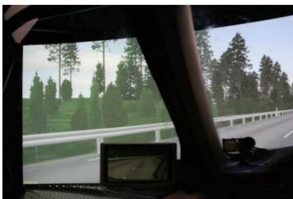
Figure 4. (a) VTI moving-base driving simulator. (b) simulator vehicle chassis (Volvo 850). (c) wide-angle visual screen with 120° horizontal field of view. (d) visual projection system. (e) left outside mirror (monitor). (f) rear mirror (monitor) and right outside mirror (monitor).
