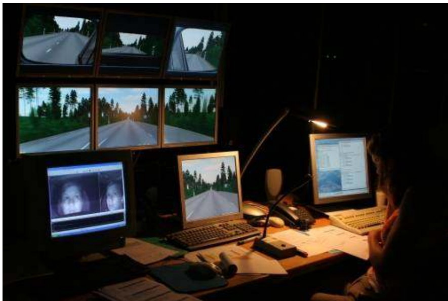
Figure 21. Desk of the experimental leader during the experiment. The experimental leader did supervise the proper progress of the study and the participants' behaviour via multiple monitors. Participants could at any time talk to the experimental leader via a microphone.
