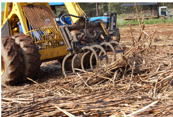
(a) A Bell loader grabs and collects cane from a windrow.
