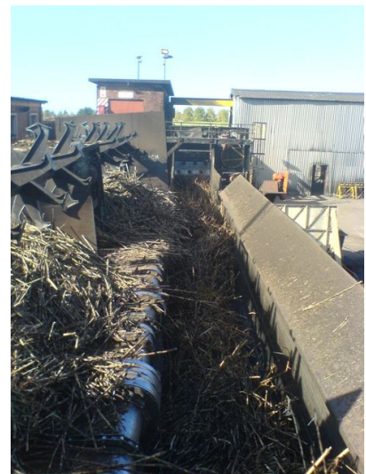
(b) Spiller table buffering the cane before the shredder.
