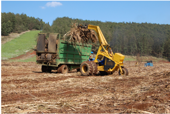
(a) Unloading onto a tractor-trailer combination.
