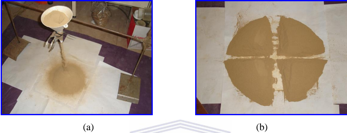
Figure 2-19: (a) Coning process (b) a quartered sample.
