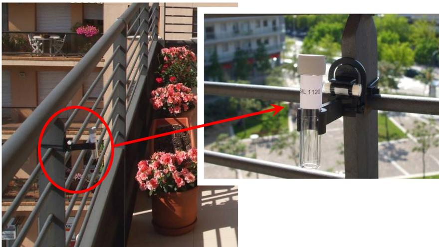
**Figure 8.** Picture of the NO<sub>2</sub> passive sampler set outdoor of participant's homes
