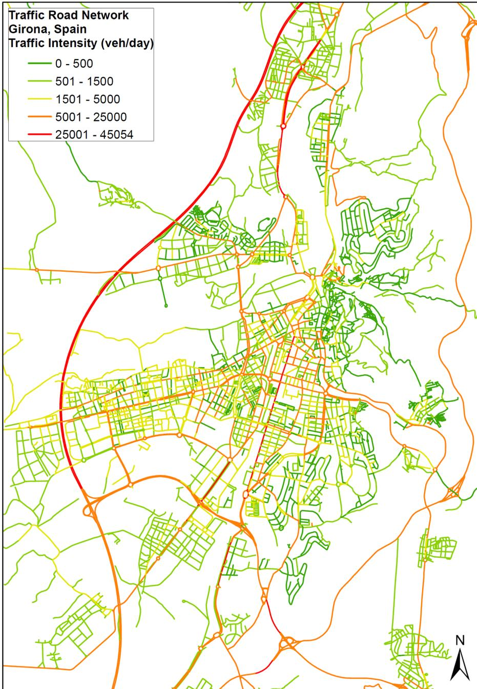
**Figure 12.** Traffic intensity road network database. Area shown: Girona city and Salt.
