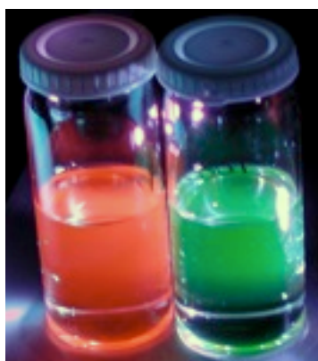
Figure 2. Digital picture of CdSe colloidal quantum dots prepared at ICIQ of different size illuminated with UV light.
