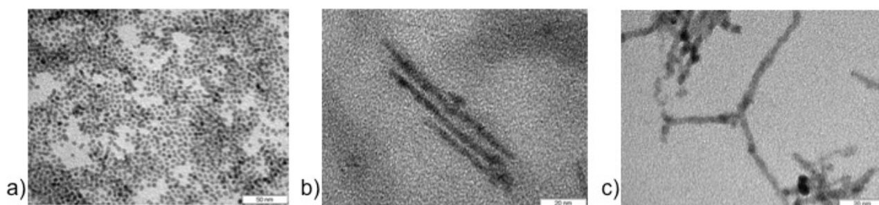
Figure 24. TEM images of CdSe quantum dots (a), nanorods (b) and tetrapods (c).
