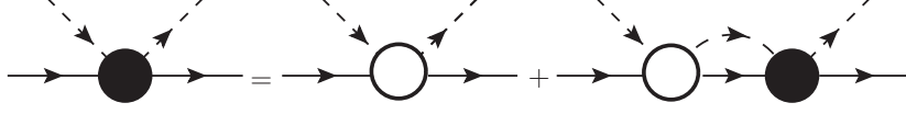
Figure 2.3: Diagrammatic representation of the Bethe-Salpeter equation. The black area corresponds to the T_{ij} matrix and the open circles correspond to the kernel V_{ij} .
