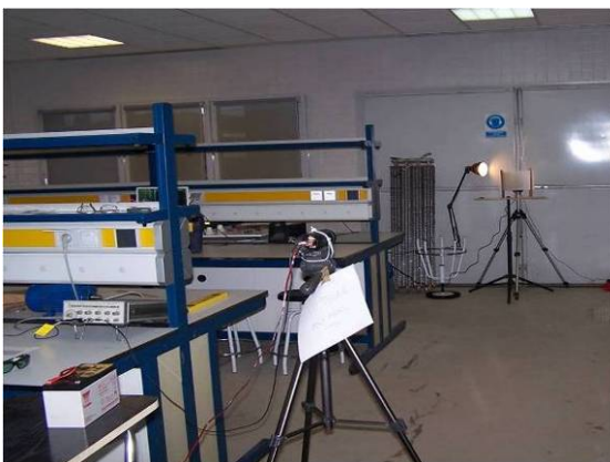
General view of the test set-up for emission characterisation: the laser emitter can be seen in the foreground and in the background is the screen which intercepts the infrared beam. Behind the screen is the infrared camera which records the beam spot image.
