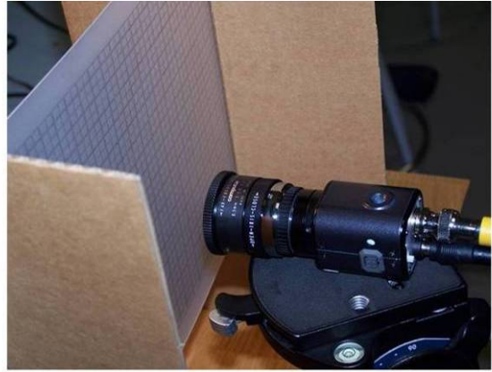
Detail of the infrared camera used to record the image of the laser beam section when striking the translucent paper screen.
