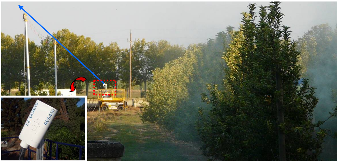
Fig. 1.1. Elastic lidar system (in the background, Leosphere ALS 300) measuring the drift generated by a hydropneumatic sprayer (behind the trees) treating an apple orchard on 24/09/2009 in Gimeneils (Lleida). In the bottom left-hand corner an enlarged view is shown of the emitter/receiver unit. The blue arrow represents a recreation of the emitted UV laser beam.
