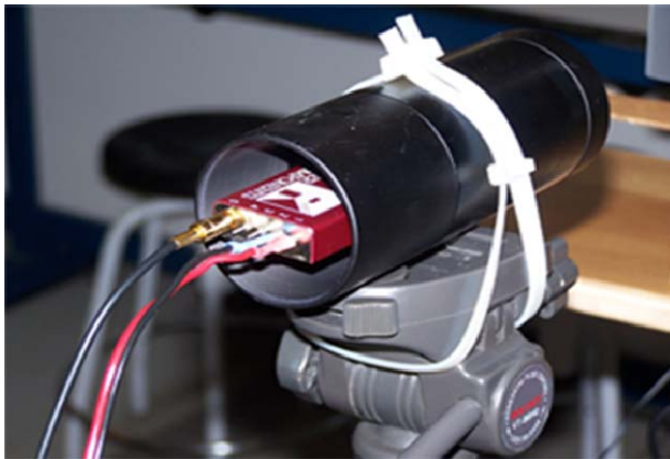
Rear view of the emitter system, showing the attachment of the laser to the expansion optics.
