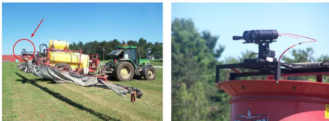
Fig. 2.6. INO Short-range lidar placed on the rear end of a hydropneumatic sprayer (Allard et al., 2007).
