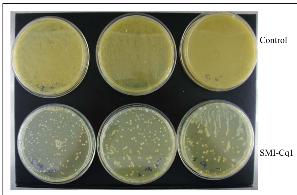
Figure 5.10: Agar plate images ( S. aureus ). Comparative view of the plated 10^{-1} diluted solutions between the control and the treated culture with SMI-Cq1 fibers.
