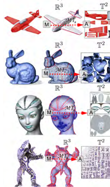
Figure 3.12: Sample models with color attributes stored in a texture atlas. The mapping \mathcal{MT}_a is an artist parameterization for attaching the shape and shading attributes to the triangle meshes.
