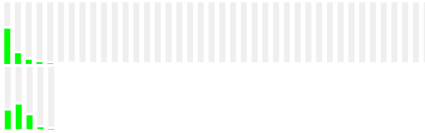
Figure 5.2: Hashing 2^{20} defined keys randomly distributed in a universe of 2^{24} keys into a hash table of 1.3 million keys (the load factor is 0.8). Histogram of insertion ages for open addressing (top) and Robin Hood (bottom). Gray bars correspond to very few items but are non-zero. The maximum age goes down from 46 to only 5.
