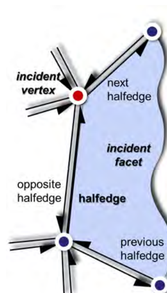
Figure 2.10: Half-edge mesh data structure: one incident face (shown in light blue) and one incident vertex (shown in red) are stored for each half-edge.
