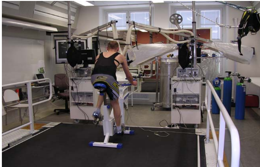
Fig. 9 Experimental setup of the Douglas Bag system and the metabolic carts used in the studies.
