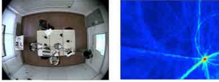
Figure 7.5: An example of TDOA trajectories in a 2D space related to the real space into the smart-room. The intersection of trajectories identify an acoustic source, in this case, a lecturer close to a blackboard. The color is related to the contribution of cross-correlation of all microphone pairs in that position. The red point corresponds to the maximization of such a cross-correlation function. Right picture courtesy of Carlos Segura Perales.
