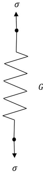
Fig. 1.8: A spring: mechanical analog to elastic behavior
