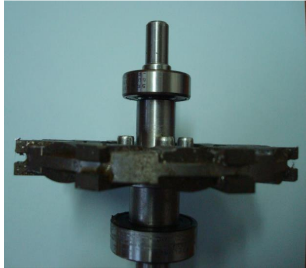
Fig. 1.7. Photograph of the PM-rotor assembly, the rotor shaft and the two bearings of different size.
