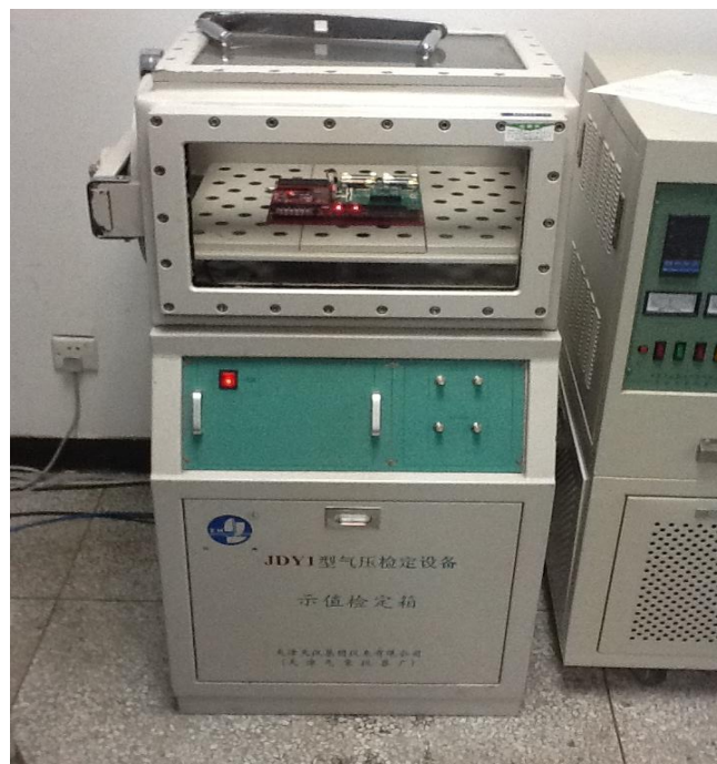
Fig. 4.15 The pressure vessel for pressure sensor testing
