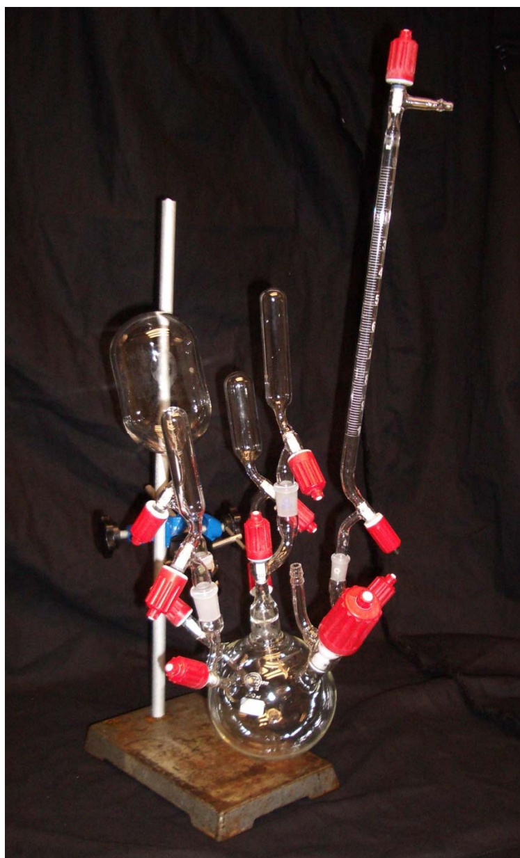
Figure 2.10. Assembled apparatus of home made high vacuum system.
