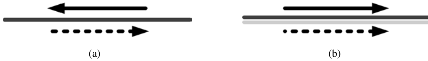
Fig 35. (a) Electric source above and its image below electric conductor (electric boundary condition). (b) Electric source above and its image below magnetic conductor (magnetic boundary condition).
