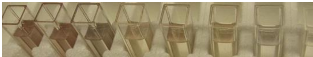
Figure 4.11. Gold nanoparticles in solution prepared simultaneously in a carousel reactor to study synthetic conditions
