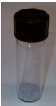
Figure 4.20. Gold nanoparticles deposited onto a silica support
