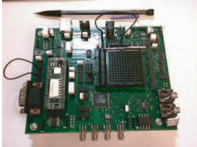
Figure 9. FPAA Programming and Control Board (25.76 square inches). Note the USB connection on the top left; 40 pin DIP microcontroller module to the right of the serial connector; the 100 pin ZIF socket for inserting the FPAA ICs; many 2x4 pin headers connected to FPAA I/O, DAC outputs, ADC inputs, FPAA control pins, and power/ground; 4 SMA for FPAA I/O interface; and the audio jacks (on the lower right).
