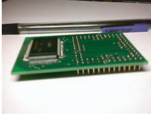
Figure 10. Adaptor Board (4.16 square inches). This custom PCB has a quad flat pack (QFP) packaged FPAA IC on one side and pins on the other side. The pins plug into the 100 pin ZIF socket on the programming and control board.
