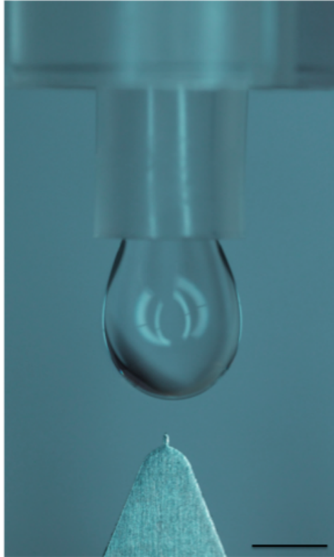
Figure 3.3.1.1. Image of microneedle used in this study. Scale bar indicates 2mm.
