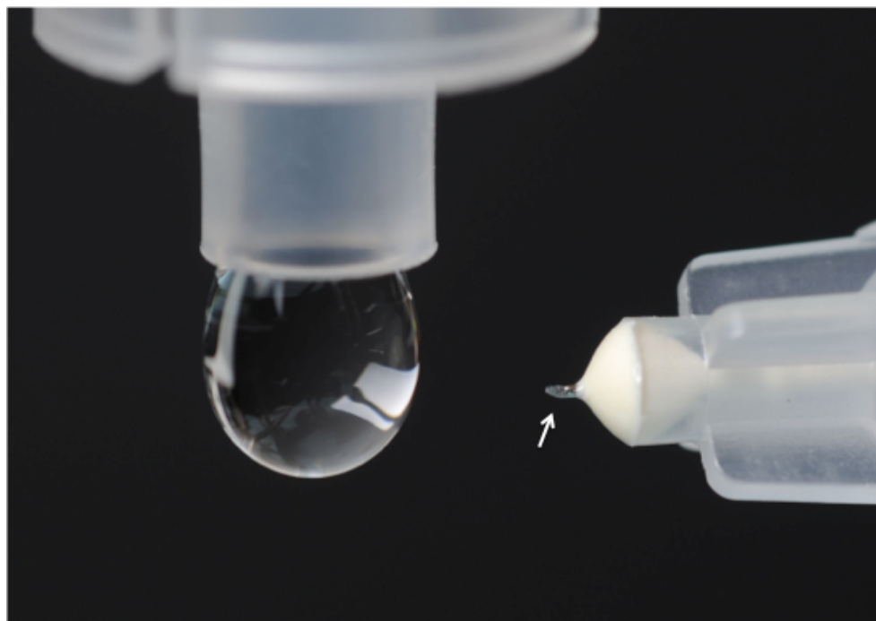
Figure 5.3.3.1. Hollow microneedle (at arrow) measuring 720 \mu\text{m} in length shown next to a liquid drop of approximately 50 \mu\text{l} volume from a conventional eye dropper.
