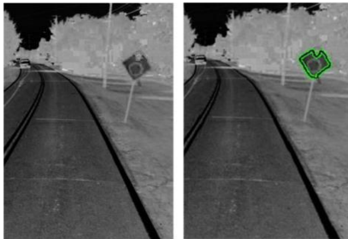
Figure 3-12 Example of a false negative case using the unconstraint active contour
