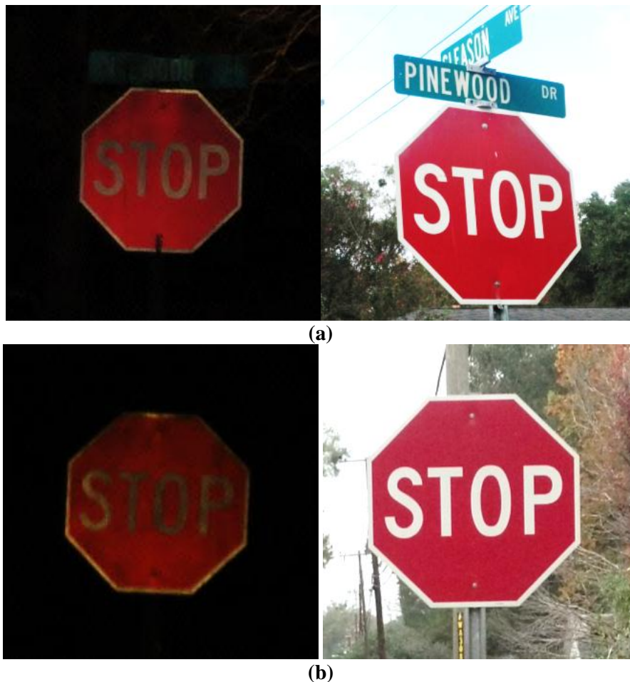
Figure 5-22 Nighttime and daytime images for (a) Sign #19 and (b) Sign #22 (Image enhanced to visualize the defects)
