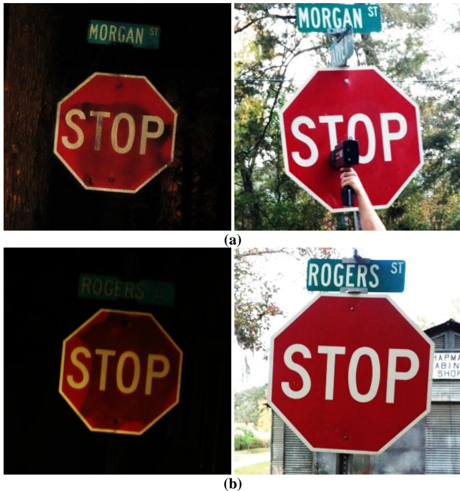
Figure 5-23 Nighttime and daytime images for (a) Sign #23 and (b) Sign #34 (Image enhanced to visualize the defects)
