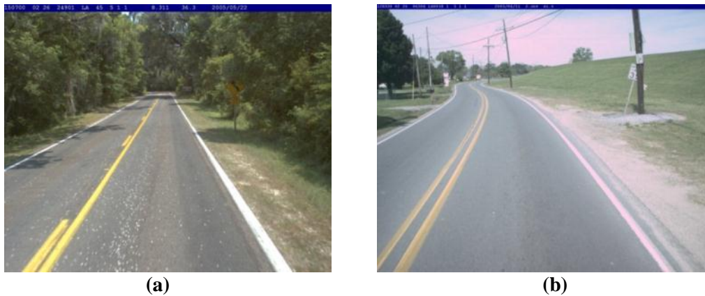
(a) (b) Figure A-5 Samples of FN cases due to occlusion a) by branches; b) by utility pole
