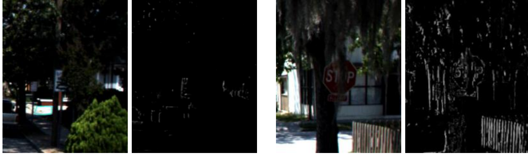
Figure 5-13 False negative cases due to occlusion (Left: original image; right: color segmented image)
