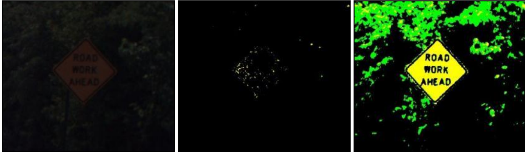
Figure 5-10 Detection results using 1) the existing algorithm and 2) the enhanced algorithm
