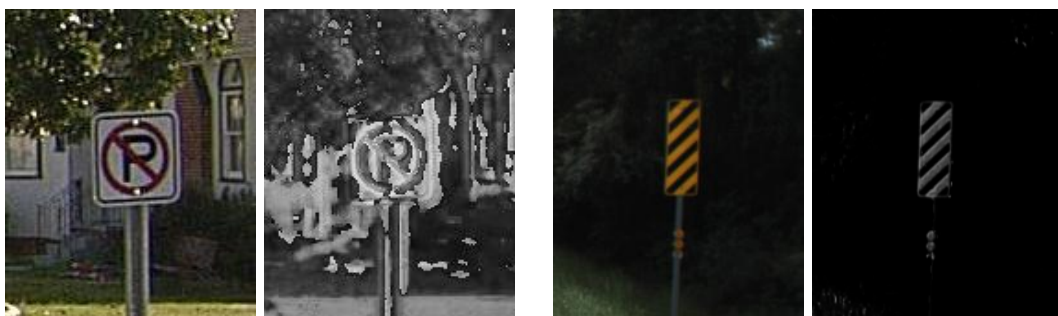
Figure 5-14 Several specific types of signs undetected (Left: original image; right: color segmented image)
