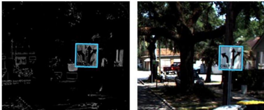
Figure 5-9 Challenging case due to the casting tree shadow (Left: color segmented image; right: original image)
