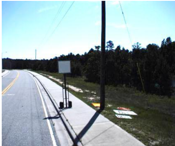
Figure 5-16 Repeatability test conducted using white Type 1 sheeting on campus
