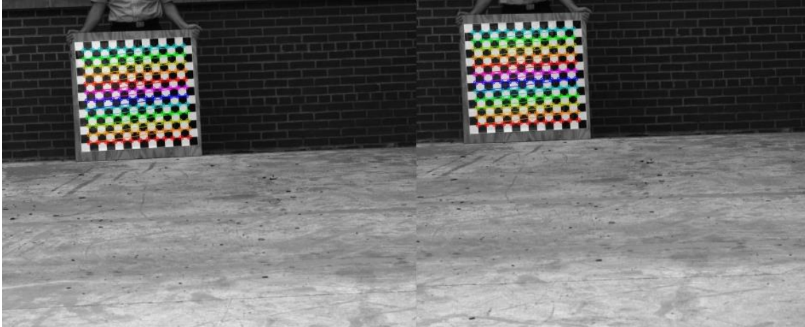
Figure 3.1: Automatically detected and matched corner points in the calibration process using OpenCV
