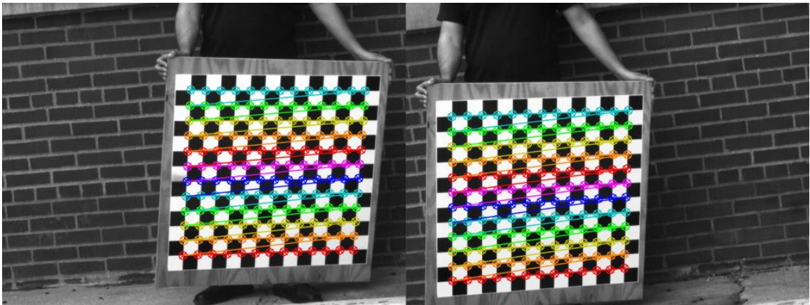
Figure 4.2: Automatically detected and matched calibration board corners
