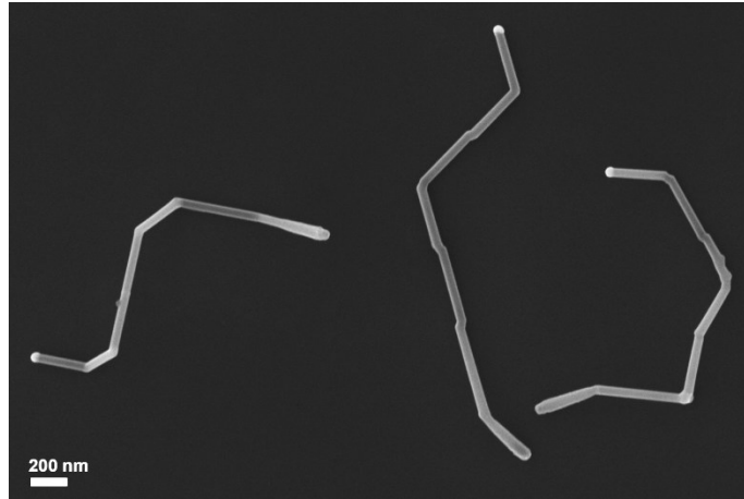
Figure 3.11 SEM image of three Ge nanowire superstructures, from the same sample as that shown in Figure 3.9b, laying side by side after sonication from the growth substrate and drop-casting onto a Si wafer.
