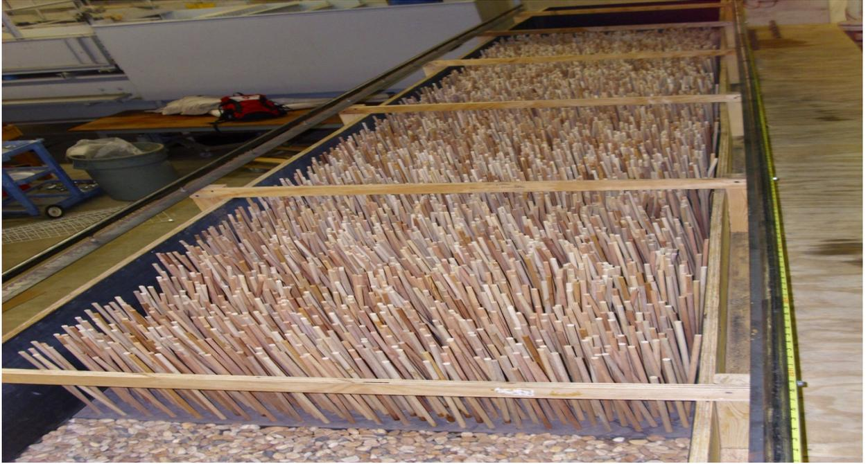
Figure A. 2: Photo of the cylindrical wooden rods simulating emergent rigid vegetation,  $m = 101.9$  stems/ft<sup>2</sup>
