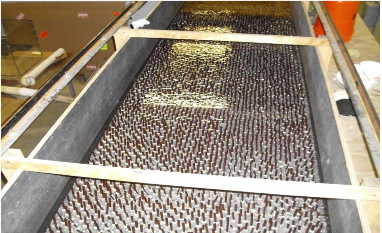
Figure A. 3: Photo of the rectangular plastic strips simulating submerged flexible vegetation,  $m = 101.9$  stems/ft<sup>2</sup>
