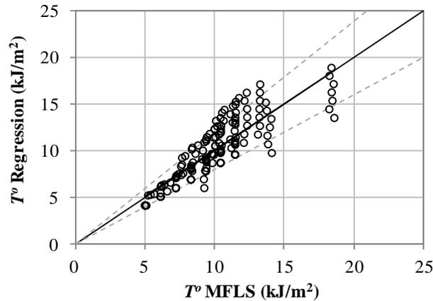
Figure 60. Comparison of  $T^0$  as calculated by the model at the multiple fiber length scale (MFLS) and regression. The solid black line represents a one-to-one relation and the dashed gray lines above and below the black line represent errors of  $\pm 20\%$ .
