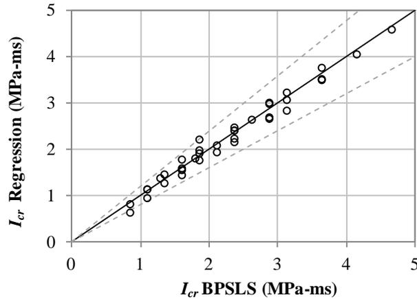
Figure 65. Comparison of the critical specific impulse  $I_{cr}$  as calculated by the Blast Panel Structural Length Scale (BPSLS) model and Equation (68). The solid black line represents a one-to-one relation and the dashed gray lines above and below the black line represent errors of  $\pm 10\%$ .
