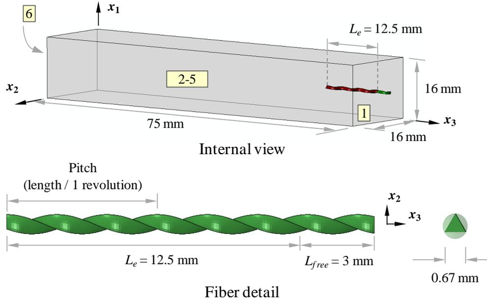
Figure 5. Illustration of the model at the internal view showing the matrix (gray), ITZ (red), and fiber (green). The  $\phi_e = 0.5$  mm triangular cross-section fiber has a pitch of 6.35 mm and total length of 15.5 mm, of which 12.5 mm was embedded into the cementitious matrix.
