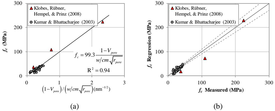
Figure 63. (a) Fitting of material constant  $K$  for the compressive strength as a function of the volume fraction of pores,  $V_{pore}$ , mean pore radius,  $r_{pore}$ , and mass ratio of water to cementitious materials,  $w/cm$ . (b) Comparison of  $f_c$  as calculated by Equation (63) to  $f_c$  as experimentally measured. The solid black line represents a one-to-one relation and the dashed gray lines represent errors of  $\pm 10\%$ .
