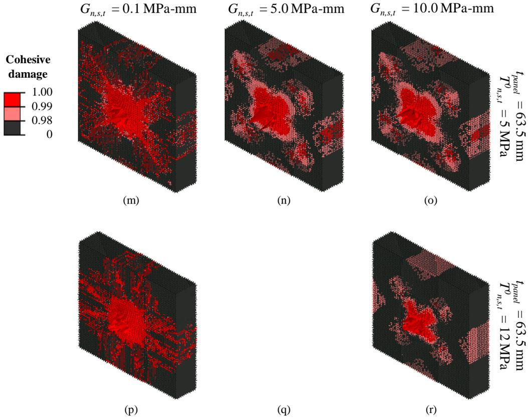
Figure 42. Cohesive damage of simulated UHPC panels 90  $\mu$ s after the impact of a projectile traveling at 1,000 m/s. The instantiations shown have material properties of  $G_{n,s,t} = 0.1, 5.0,$  and  $10.0$  MPa-mm;  $T^o = 5$  and  $12$  MPa; and  $t_{panel} = 38.1, 50.8,$  and  $63.5$  mm.
