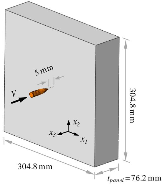
Figure 38. Model of penetration at the structural length scale.
