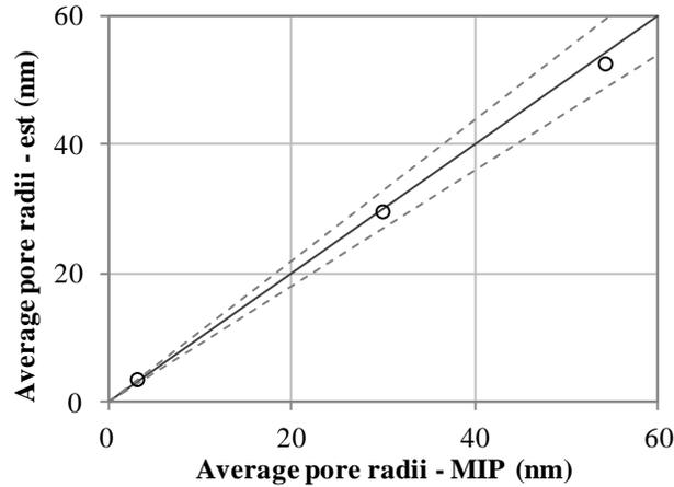
Figure 56. Comparison of average pore radii,  $r_{pore}$ , measured experimentally by Klobes et al. (2008) and estimated via MCTP model. The solid black line represents a one-to-one relation and the dashed gray lines above and below the black line represent errors of  $\pm 10\%$ .
