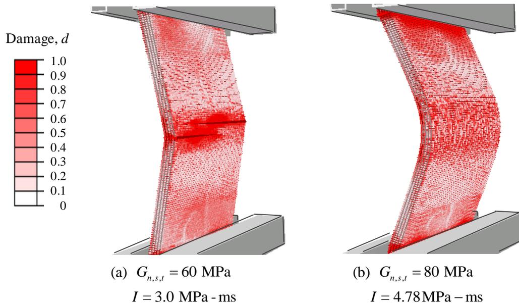
Figure 37. Comparison of damage, deformation, and fracture patterns for 63.5-mm thick simulated panels with  $T_{n,s,t}^0 = 14.7$  MPa, and (a)  $G_{n,s,t} = 60$  MPa and (b)  $G_{n,s,t} = 80$  MPa. Images are shown 12 ms after the initiation of a (a) 3.0 MPa-ms and (b) 4.78 MPa-ms applied impulse.
