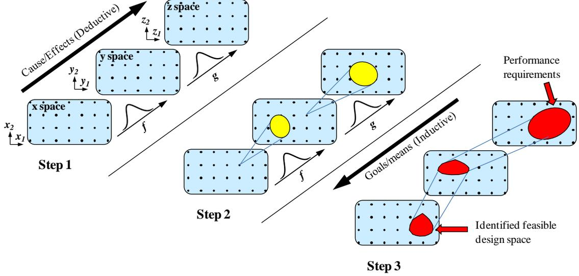
Figure 44. Schematic of Inductive Design Exploration Method (IDEM) applied to a three-space hierarchical problem consisting of  $x$ -,  $y$ -, and  $z$ -spaces. The schematic is shown with two variables in each space.
