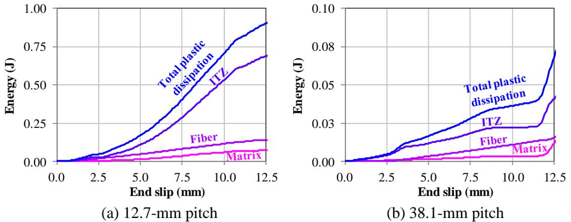
Figure 13. Partition of total plastic dissipation as a function of end slip for (a) 12.7-mm and (b) 38.1-mm pitched fibers. Each fiber was embedded 12.5 mm into an ITZ-matrix system with  $f_c = 44$  MPa.
