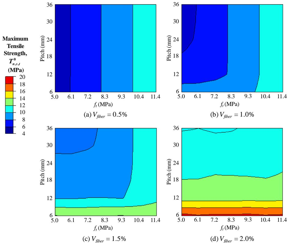
Figure 59. Maximum tensile strength as a function of fiber volume fractions between 0.5 and 2%, fiber pitch, and non-reinforced matrix tensile strength. All fibers had a 0.5-mm equivalent diameter and 25-mm length.
