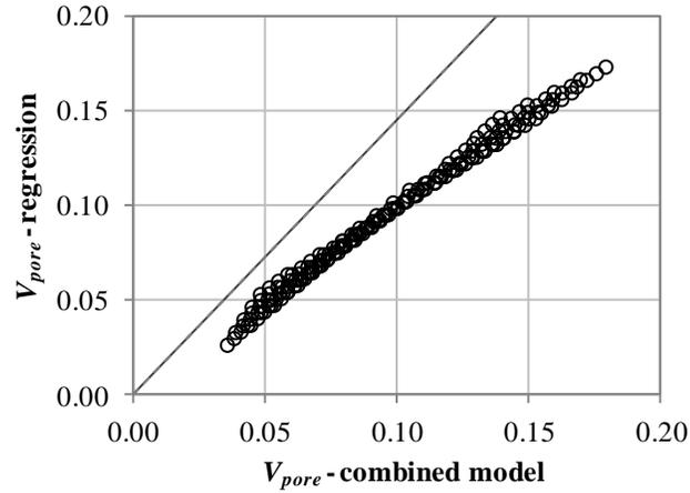
Figure 57. Comparison of  $V_{pore}$  predicted by regression model (i.e., Eq. (54)) and  $V_{pore}$  predicted by the MCTP model. The solid black line represents a one-to-one relation and the dashed gray lines above and below the black line represent errors of  $\pm 10\%$ .
