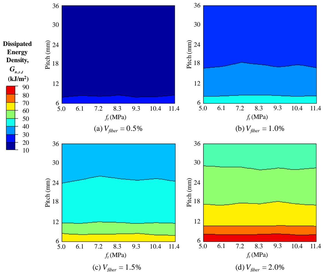
Figure 61. Dissipated energy densities as functions of fiber volume fractions between 0.5 and 2%, fiber pitch, and non-reinforced matrix tensile strengths. All fibers had a 0.5-mm equivalent diameter and 25-mm length.
