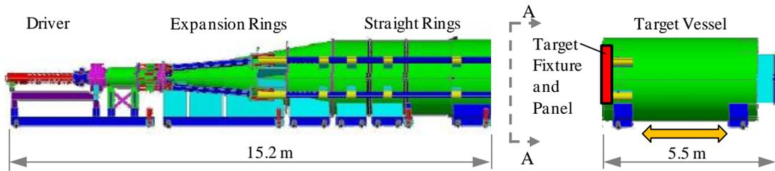
Figure 28. Schematic of Blast Load Simulator (BLS).
