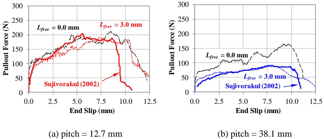
Figure 15. The effect of free length of fiber quantified by the pullout force as a function of end slip for initial fiber pitches of (a) 12.7 mm and (b) 38.1 mm embedded in a  $f_c = 44$  MPa matrix. Experimental data of Sujivorakul (2002) show as solid lines; numerical simulation data with  $L_{free} = 3.0$  mm shaded the same color as the experimental data with dashed lines; numerical simulation data with  $L_{free} = 0.0$  mm are shaded as black dashed lines.
