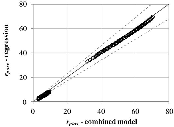
Figure 58. Comparison of  $r_{pore}$  predicted by regression model (i.e., Eq. (55)) and  $r_{pore}$  predicted by the MCTP model. The solid black line represents a one-to-one relation and the dashed gray lines above and below the black line represent errors of  $\pm 15\%$ .
