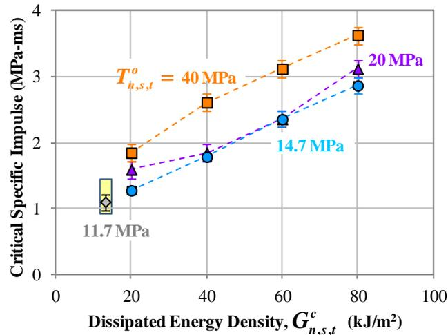
Figure 35. Calculated critical specific impulses required to completely fracture the simulated UHPC panel with dissipated energy densities between 20 and 80  $\text{kJ/m}^2$  and tensile strengths of 14.7, 20, and 40 MPa.
