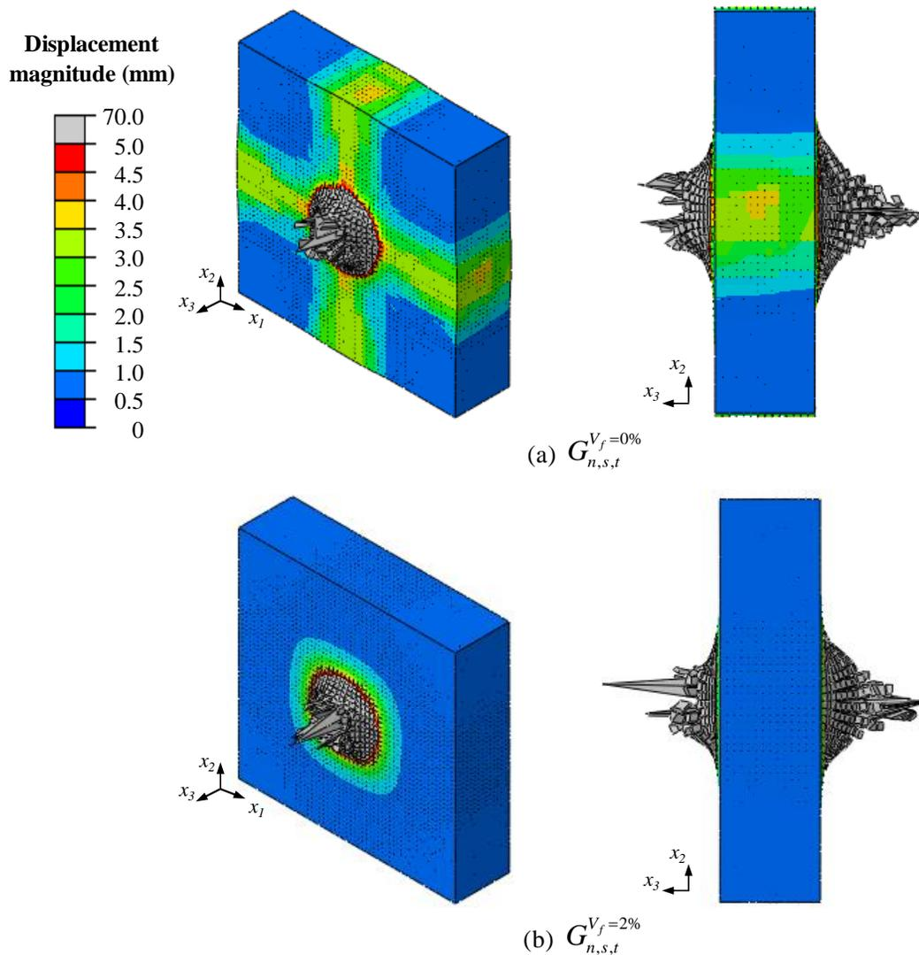
Figure 40. Displacement magnitudes for UHPC panels reinforced with (a)  $G_{n,s,t}^{V_f=0\%}$  and (b)  $G_{n,s,t}^{V_f=2\%}$  of 0.185-mm diameter by 14-mm long steel fibers. Images are shown 150  $\mu$ s after impact of a projectile with a velocity of at 914 m/s.
