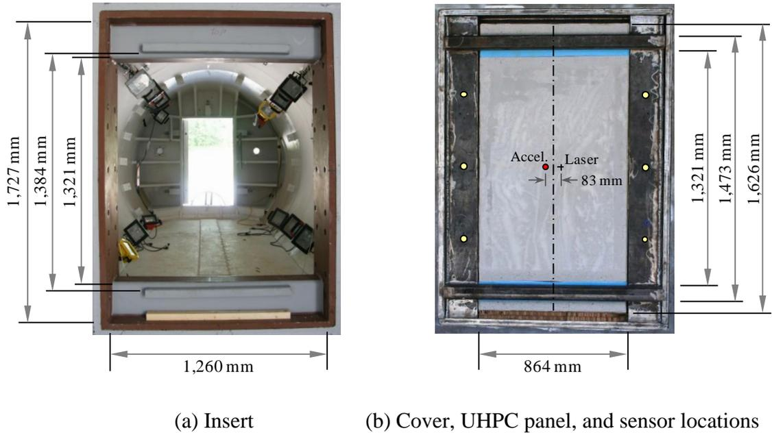
Figure 29. Target fixture as viewed from section A-A (cf. Figure 28) showing the (a) target fixture insert and (b) target fixture cover, proximal face of UHPC panel, and sensor locations.
