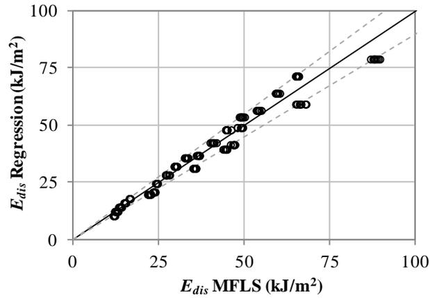
Figure 62. Comparison of  $E_{dis}$  as calculated by the model at the multiple fiber length scale and the fitting linear regression. The solid black line represents a one-to-one relation and the dashed gray lines above and below the black line represent errors of  $\pm 10\%$ .
