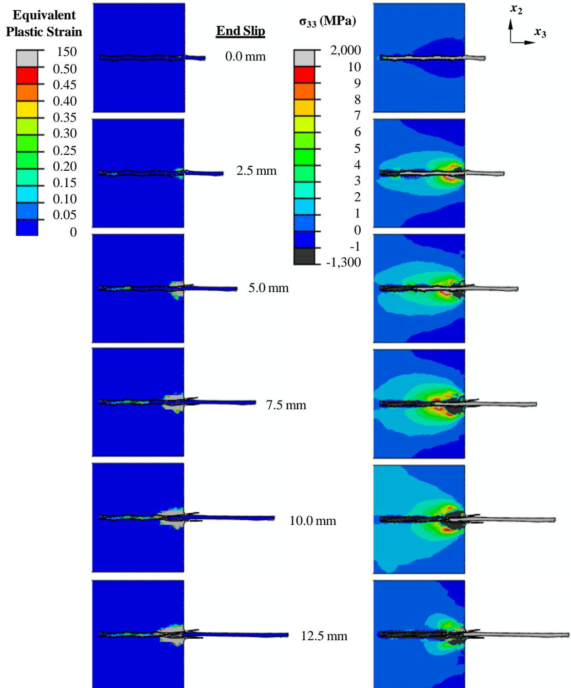
Figure 11. Evolution of equivalent plastic strain and  $\sigma_{33}$  as a function of end slip in the fiber-ITZ-matrix system. The fiber has a triangular cross section with a pitch of 12.7 mm and an embedded length of 12.5 mm in a  $f_c = 44$  MPa matrix.
