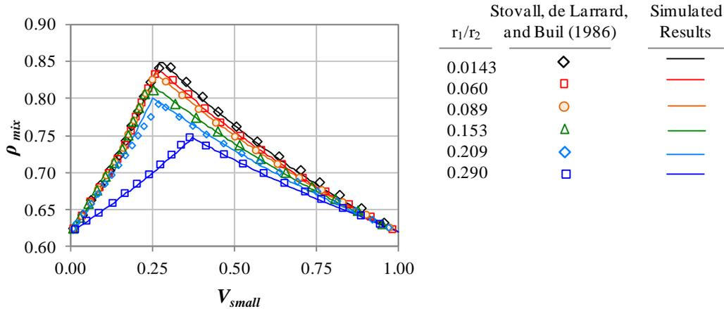
Figure 55. Comparison of simulated  $\rho_{mix}$  for a binary system of particles. Data points were reported by Stovall, de Larrard, and Buil (1986); data used to construct the solid lines were generated by the model described in Section 6.3.2.3.
