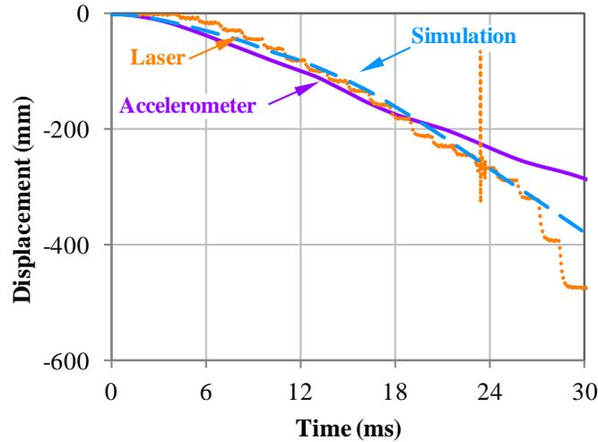
Figure 33. Comparison of displacement of the center of the panel in the  $x_3$  direction (cf. Figure 24) measured by accelerometer and laser interferometer measurement systems and the displacement predicted by the multiscale model ( $I = 2.05$  MPa-ms).
