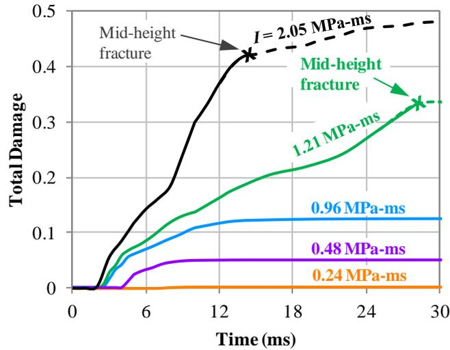
Figure 34. Total damage for simulated UHPC panel with a mean 11.7-MPa mean  $T_{n,s,t}^o$  and 13.5-kJ/m<sup>2</sup> mean  $G_{n,s,t}^o$  for impulses between 0.24- and 2.05-MPa-ms.
