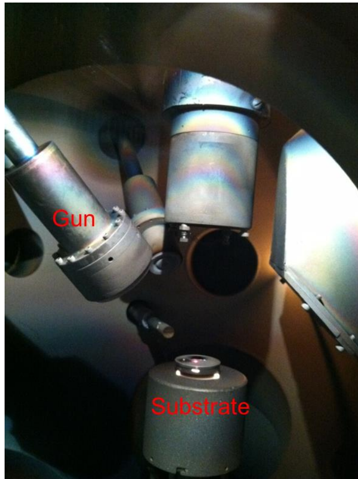
Figure 4.1 Picture of inside of deposition chamber. The sample substrate sits on a rotating stage that is heated from the backside with a tungsten filament.
