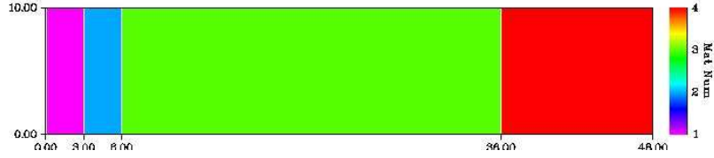
Figure 49: Fixed Source Slab Model Problem Coarse Mesh Cells, Numbered 1 to 4, left to right
