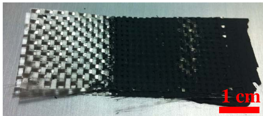
Figure 26. Experimental setup for preparing sample (top) and actual photograph (bottom) of OCNF/glass fiber assembly. Images were published in [95].
