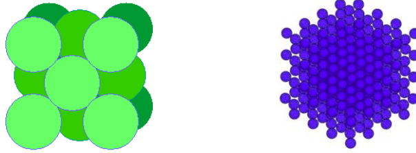
Figure 2.2: (a) Schematic of the face-centered cubic (FCC) crystal structure; (b) super cell of aluminum (Puri 2008).
