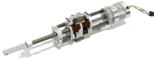
Figure 3: Series elastic actuator example.
