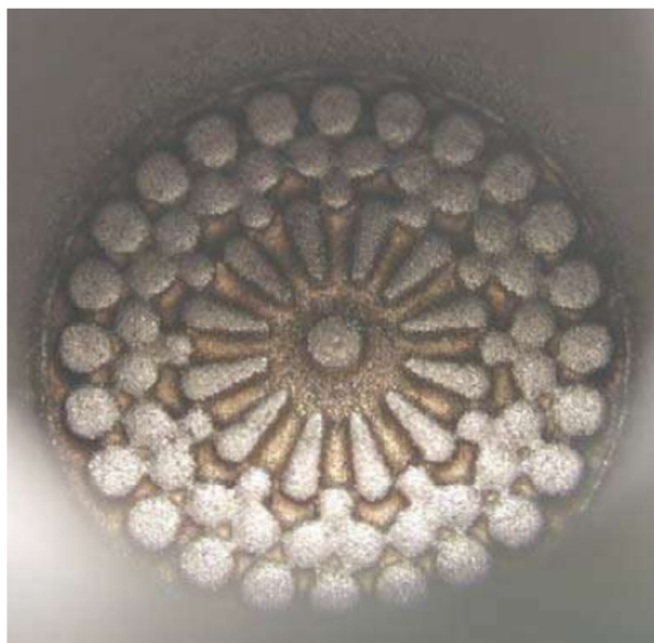
Figure 18. Attempt to EDM HEMP fin array in tungsten alloy. [8]
