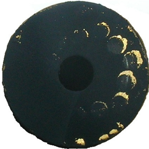
Figure 104. Photograph of sooted tube tip after compressing onto fin tips.
