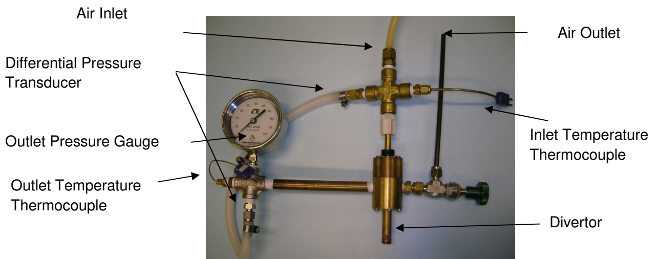
Figure 32. Picture of experiment in forward flow configuration removed from insulation.
