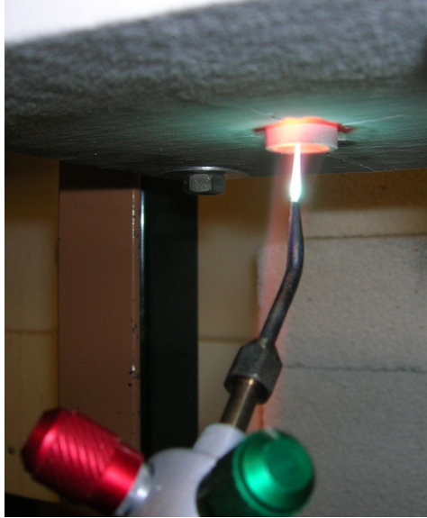
Figure 34. Test section being heated by torch. Ceramic sleeve is glowing red hot.
