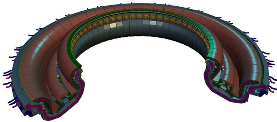
Figure 3. Cutaway view of the ITER divertor system. [2]
