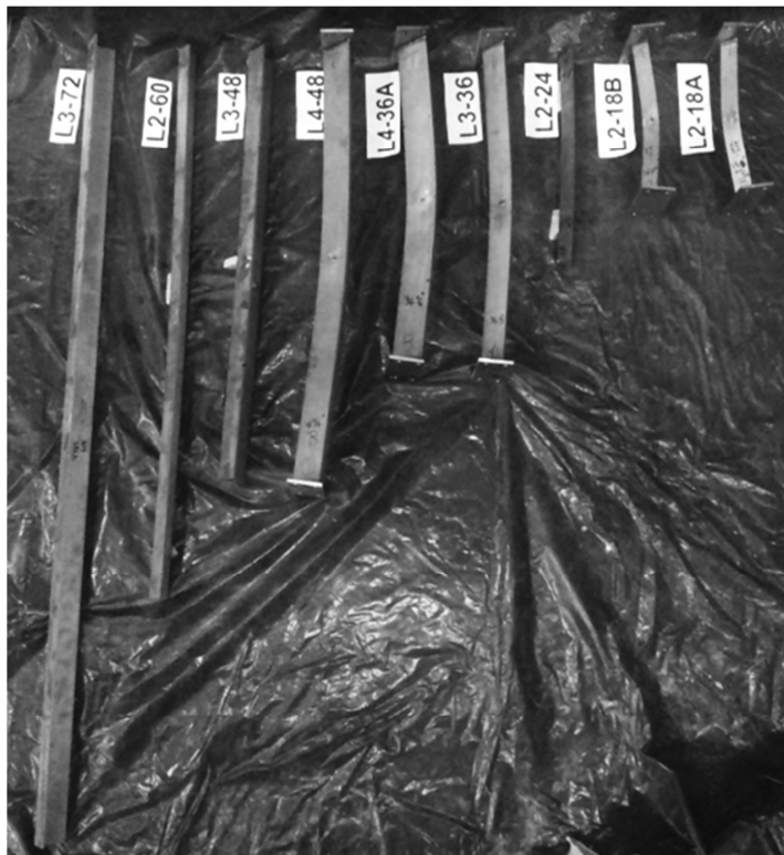
Figure 4.12- Flexural buckling specimens
