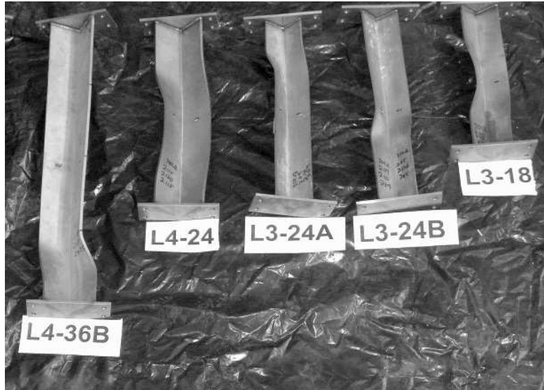
Figure 4.13- Flexural-torsional buckling specimens
