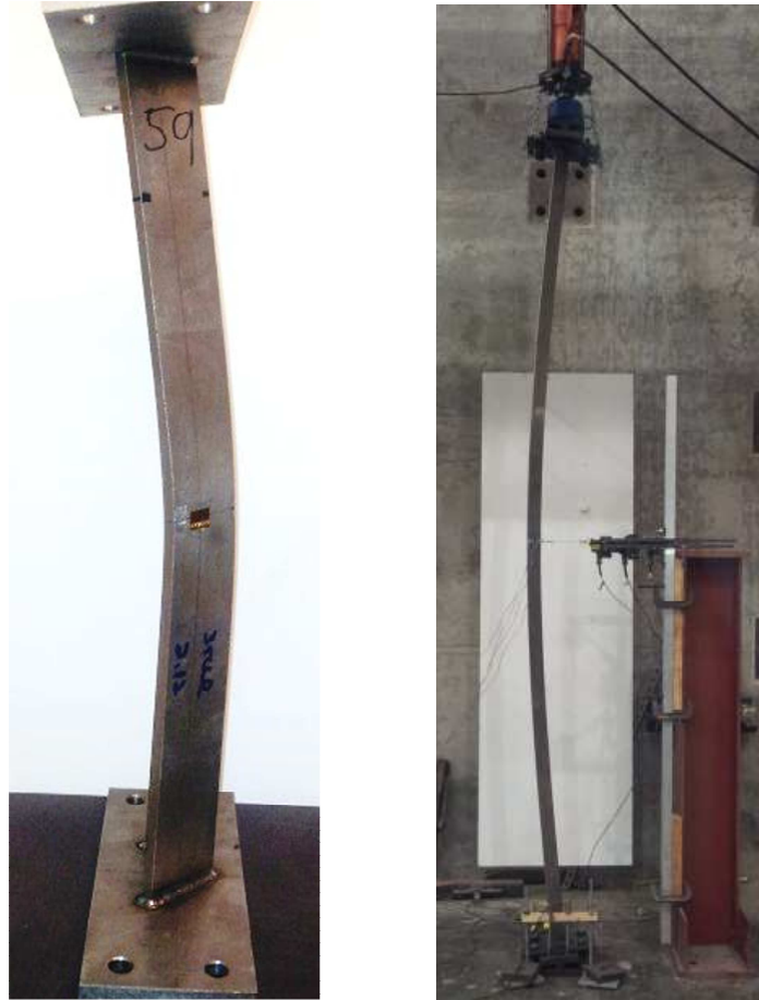
Figure 4.17- Deformed flexural-buckling specimens: L2-18a (left), L3-132 (right)
