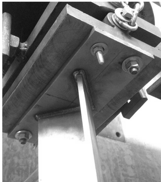
Figure 4.8- Angle endplate weld
