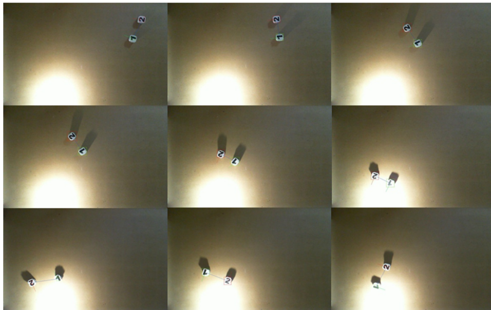
Figure 7: Snapshots of the trajectories of two agents seeking a light source.
