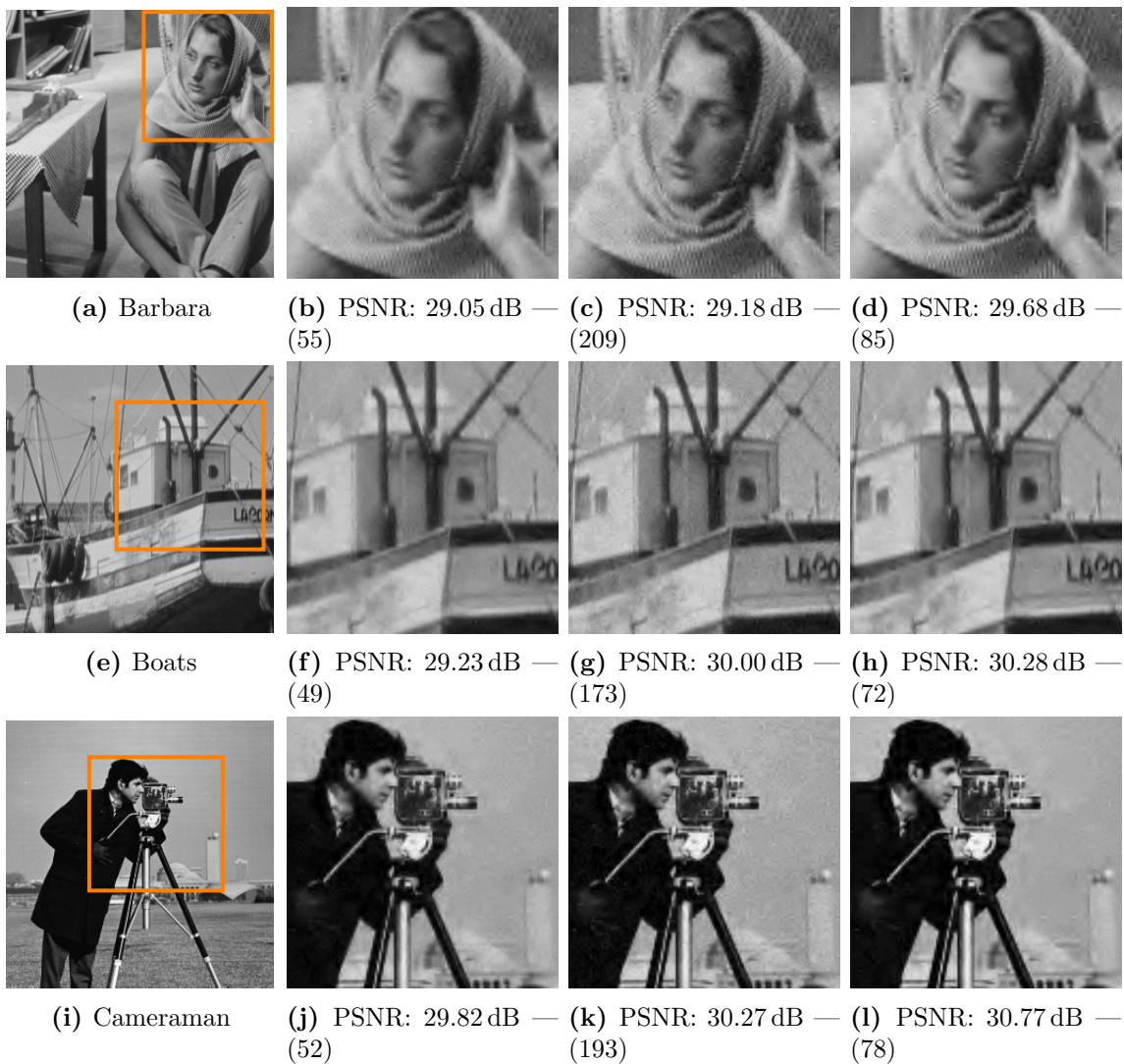
Figure 6.9: Results for the recovery of 256 \times 256 images from M = 30,000 noiselet measurements in the presence of Gaussian noise at 40dB SNR, using Daubechies 9/7 biorthogonal wavelet transform with odd-symmetric extensions as the sparse representation. (Column 1) Original images. (Column 2) Portions of the images (inside the orange box) reconstructed by solving (3.3) using SpaRSA. (Column 3) Reconstruction after three reweighting iterations. (Column 4) Adaptive reweighting by updating the w_i after every continuation step in SpaRSA. The caption under each subimage shows the PSNR over the entire reconstructed image and a count for the number of applications of \Phi^T \Phi (in parentheses) averaged over 10 experiments.
