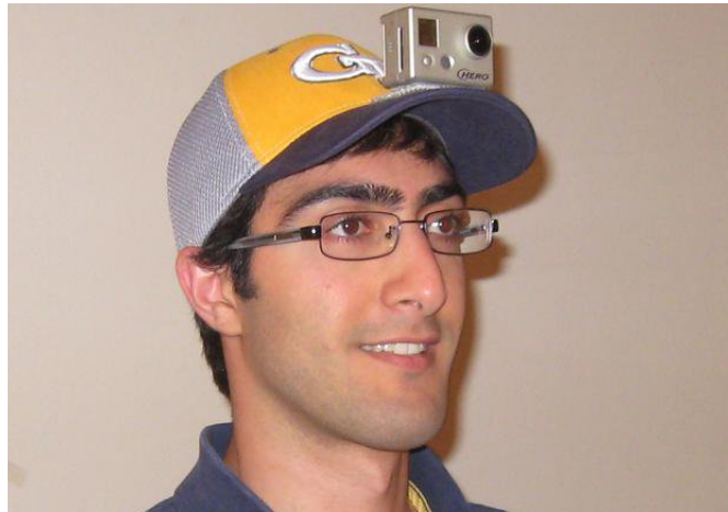
Figure 7: We used GoPro for collecting the GTEA dataset [56] and the Social Interaction at Disney park dataset [51]. We created a simple wearable device by mounting a GoPro camera on a cap using velcro tapes.
