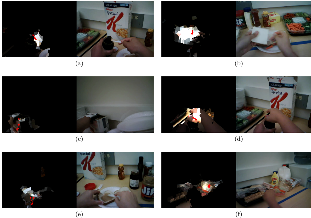
Figure 61: Our method predicts fixation locations in images for each particular action. The right hand side pictures show the frame and the left hand side images show our prediction results. The brighter the pixels are it means the higher the score returned by our algorithm is. The red dots show the ground-truth gaze locations from few adjacent frames. The actions are (a) scoop jam using knife, (b) open cheese, (c) take knife and (d) open jam, (e) spread peanut on bread using knife and (f) take bread.
