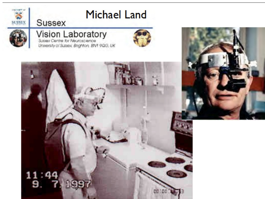
Figure 6: Michael Land used a wearable device that recorded the scene in front of the user and would measure the point of the gaze.
