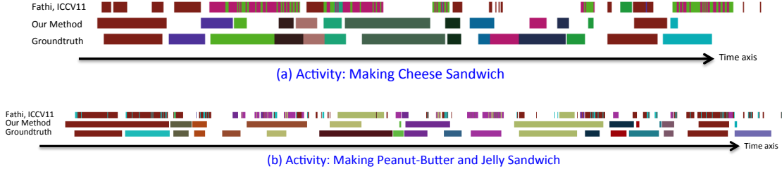
Figure 51: Activity segmentation results are shown for two test activity videos. The horizontal axis represents time (frames). Different colors represent different action labels assigned to the frames. In each example, the bottom row shows the ground-truth results, the top row shows the results of our method in Chapter 7, and the middle row shows our current results. We correctly assign true labels to 42% of frames and outperform our previous results with 33% accuracy. In addition, our labels are smoother in comparison to our previous method.
