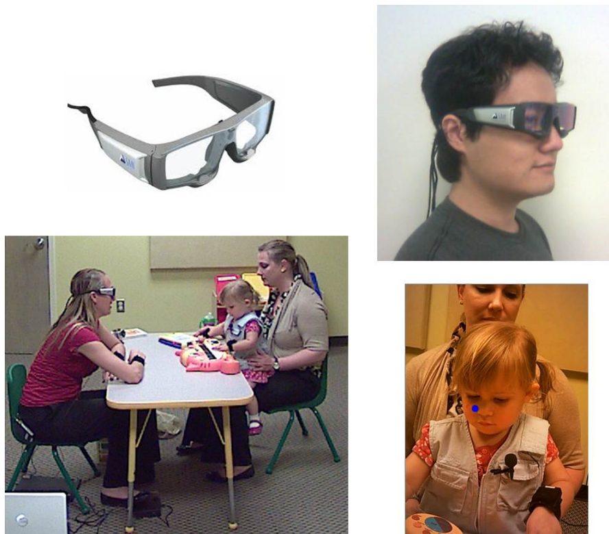
Figure 12: Experiment setup of our method. The examiner wears the SMI glasses and interacts with the child. The glasses are able to record the egocentric video with the gaze data. This figure is generated by Yin Li.
