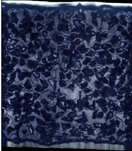
**Figure 4.8 - Stitched surface image of 0.5mm OD, #200 grit diamond grinding wheel composed from 61 individual images**
