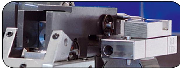
**Figure 1.7 – Difficulties in machining HAR micro-features are currently addressed using complicated fixturing techniques to support the workpiece [19]**
