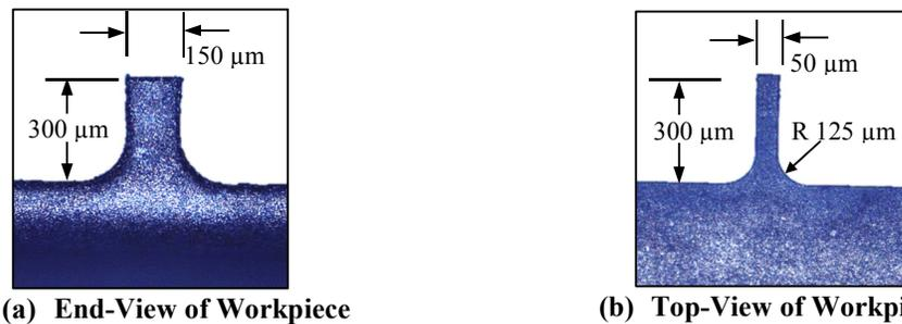
**Figure 7.9 – Micrographs of WC workpiece micro-pin features with a 150 $\mu\text{m}$  engagement width in the circumferential direction (a) and a 50 $\mu\text{m}$  engagement width in the axial direction (b) of the grind wheel**
