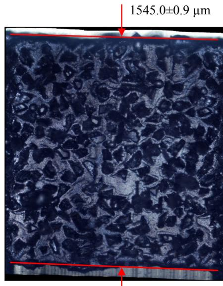
**Figure 4.13 - Inspection measurement of #200, 508μm wheel stitched surface image**
