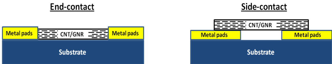
Figure 1.2 “End-contact” and “Side-contact” device configuration for carbon-based electronics
