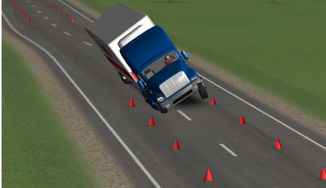
Figure 2.2: An example of an AHV rollover during a single lane change of a tractor and semitrailer combination
