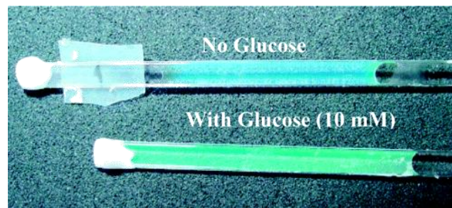
Figure 2.5. Glucose sensing microgel colloidal crystals with and without glucose. 58
