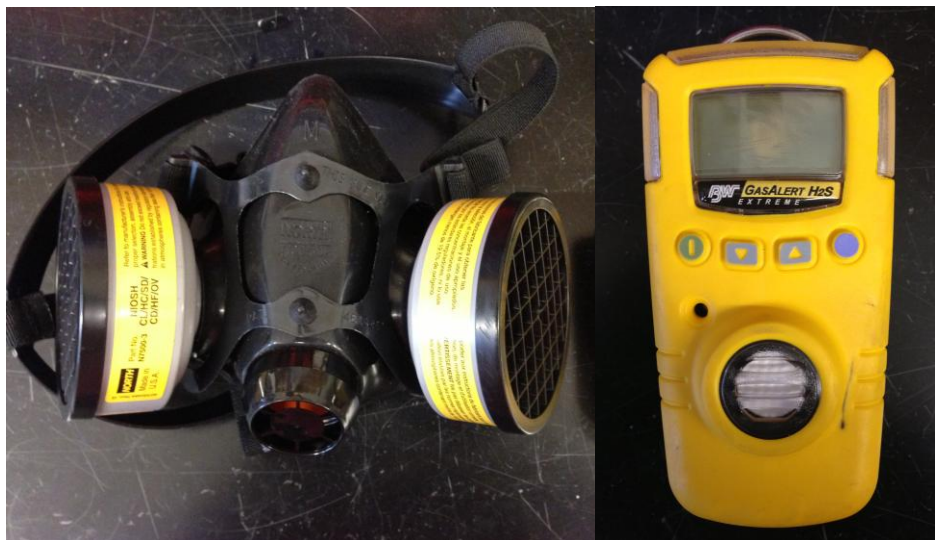
Figure 3.3: Half-mask APR respirator (left) and H 2 S detector (right) used in this study.
