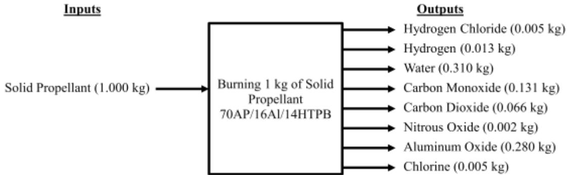
**Figure 25: Mass flows associated with burning 1 kg of a solid propellant made up of 70% AP, 16% Al, 14% HTPB**
